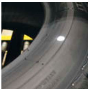
High-point marking on automobile tires
